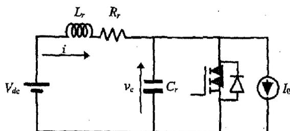
FIG. 1. Equivalent circuit of RDCLI.
