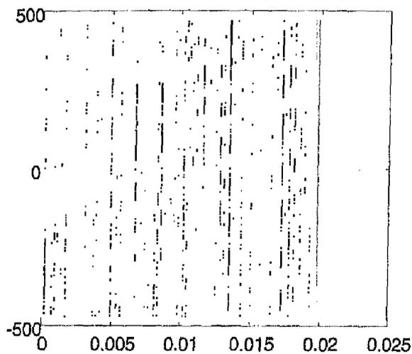
FIG. 12. PWM inverter voltage waveform for the case of Fig. 11.
