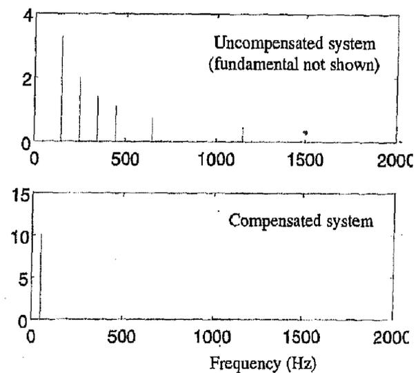
FIG. 13. Spectral performance for PWM inverter based AHCC.
