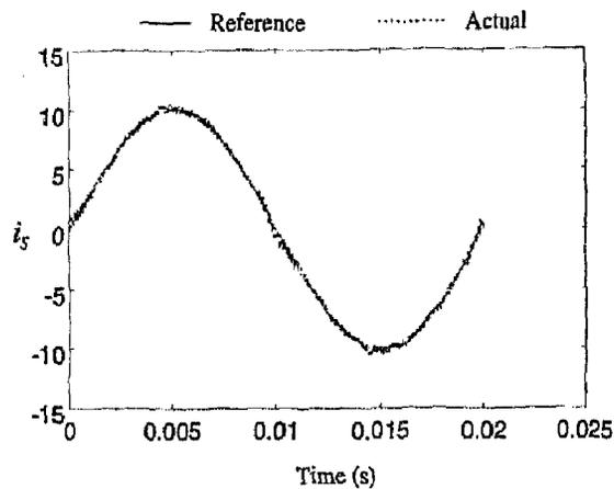
FIG. 8. Compensator performance for  $V_{dc}$  of 470 V and link frequency of 40 kHz.
