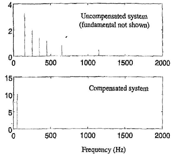
FIG. 9. Spectral performance of the compensator for  $V_{dc}$  of 470 V and link frequency of 40 kHz.
