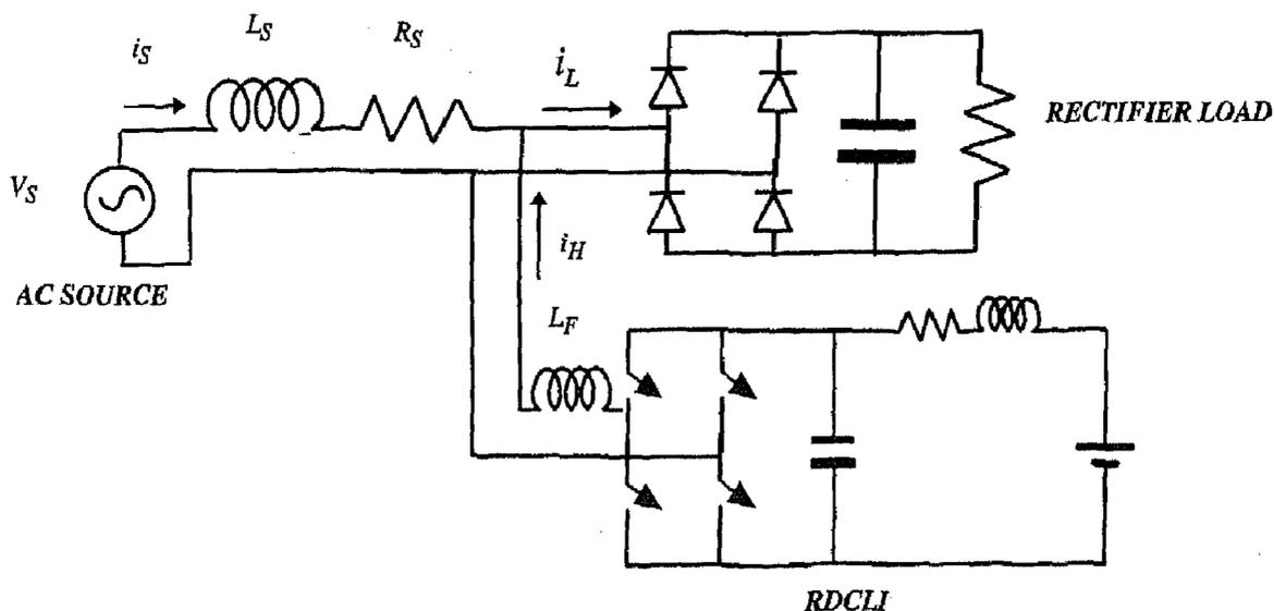
FIG. 2. Schematic diagram of the current compensating scheme.
