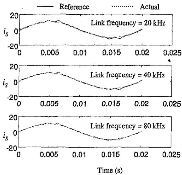
FIG. 6. Effect of link frequency variation on compensation.
