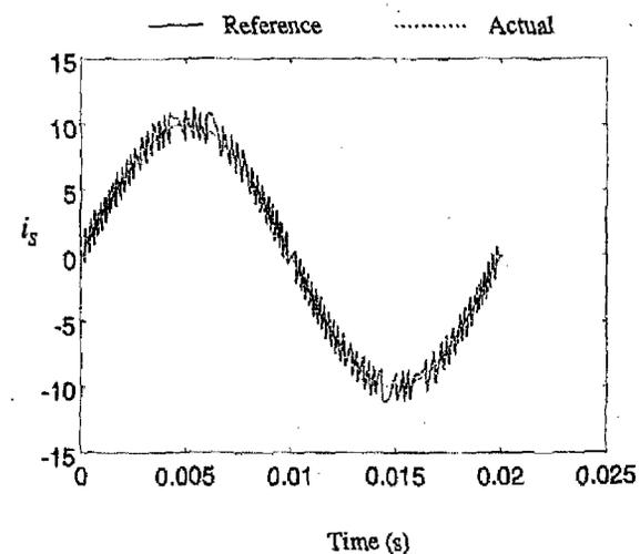
FIG. 11. Reference current and compensated current from source for a PWM inverter based compensator working at  $V_{dc} = 470$  V and average switching frequency of 8 kHz.
