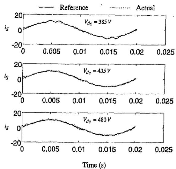
FIG. 7. Effect of dc source voltage variation on compensation.
