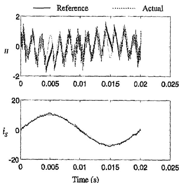
FIG. 4. Compensator current and compensated current from source in the presence of 13th harmonic.
