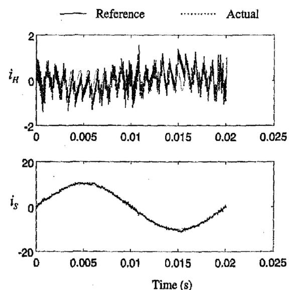
FIG. 5. Compensator current and compensated current from source in the presence of 23rd harmonic.
