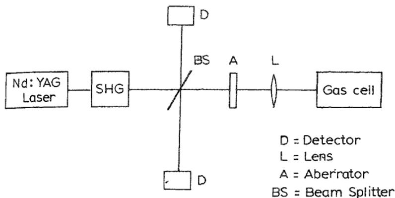
Fig. 1. Experimental layout for OPC-SBS.
