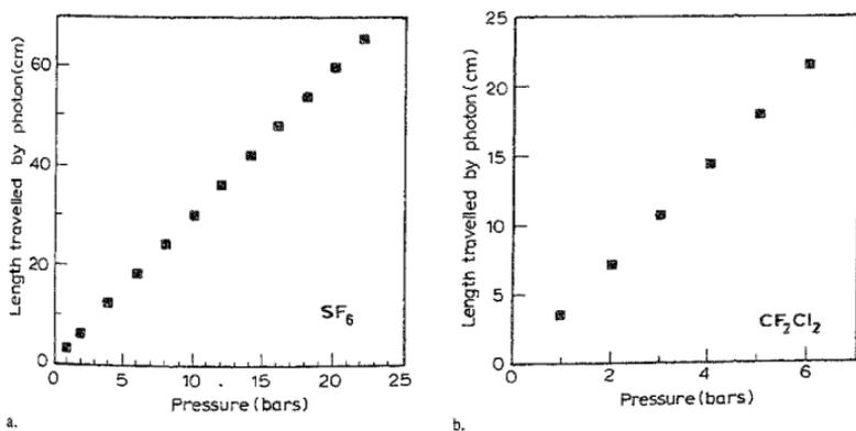
Fig. 2. Distance travelled by a photon during the lifetime of acoustic phonon. (a)  $SF_6$  and (b)  $CF_2Cl_2$ .
