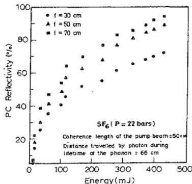
FIG. 5. Dependence of phase conjugate reflectivity on interaction length in narrow band regime when  $L_c < c\tau_{ph}$  ( $L_c = 5$  cm).
