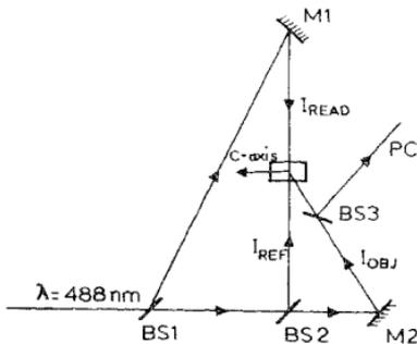
FIG. 1. Experimental FWM scheme to generate phase conjugate waves.
