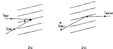
FIG. 2. Schematic representation of four-wave mixing as lapsed-time holographic process.
