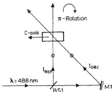
FIG. 3. Two-beam coupling scheme to generate forward phase conjugate wave. The input waves are polarized normal to c-axis.
