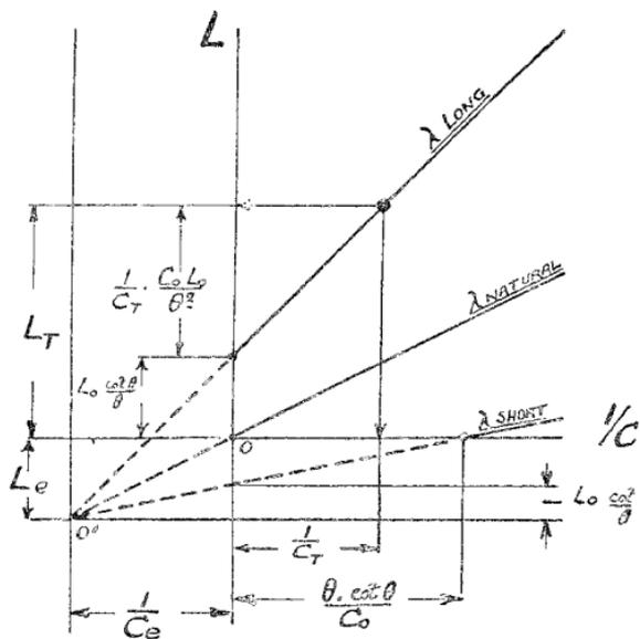
Fig. 1. Analysis of Characteristics.
