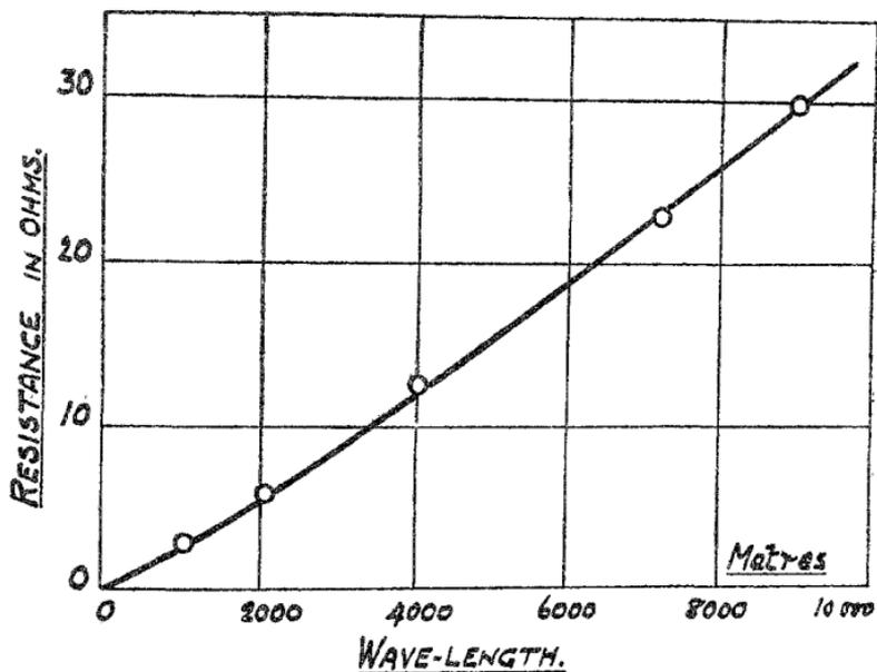
**Fig. 9.** Variation of Dielectric Resistance with wavelength.
