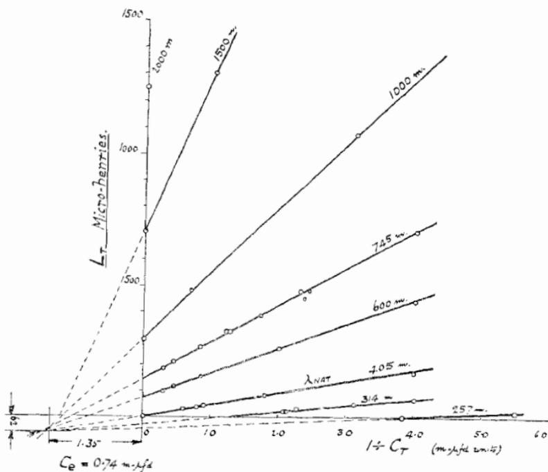
**Fig. 2.** Tuning Characteristics of Small Aerial with Counterpoise.
