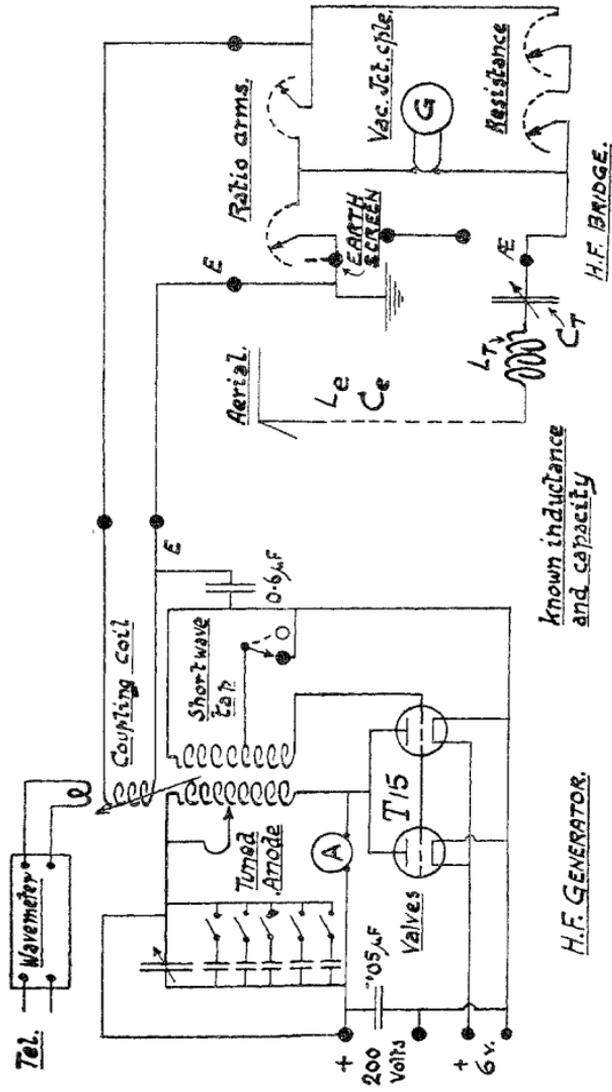
**Fig. 6.** 30-Watt H.F. Generator and Aerial Testing Bridge with Wavemeter.
