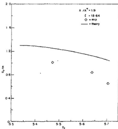
FIG. 6. Variation of small-signal gain with the universal parameter  $\chi_1$  for the composition CO<sub>2</sub>:N<sub>2</sub>:He = 12.49:39(%).
