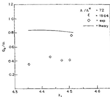
FIG. 8. Variation of small-signal gain with the universal parameter  $\chi_1$  for the composition  $\text{CO}_2\text{:N}_2\text{:He}=15.25\text{:}60(\%)$  at different locations in the nozzle
