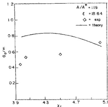
FIG. 7. Variation of small-signal gain with the universal parameter  $\chi_1$  for the composition  $\text{CO}_2\text{:N}_2\text{:He}=15\text{:}25\text{:}60(\%)$ .
