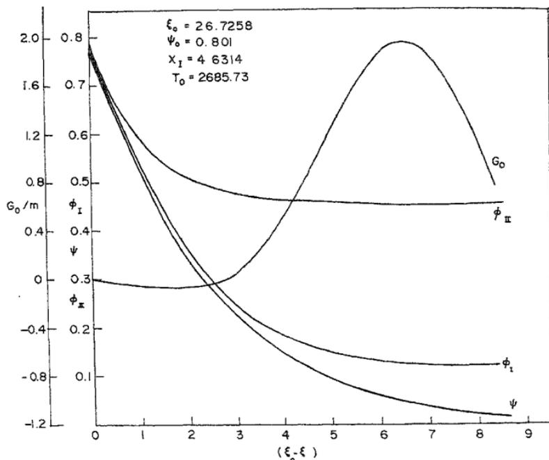
FIG. 4. Variation of the temperatures and the small-signal gain along the nozzle axis.
