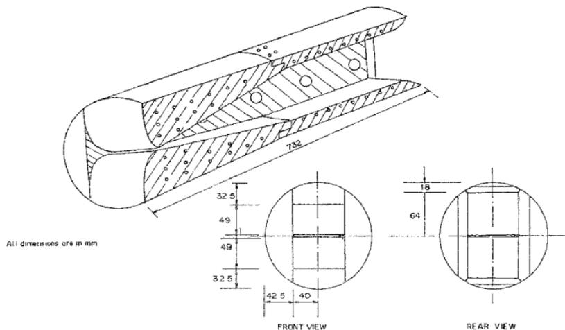
FIG.2. Design details of the two-dimensional wedge nozzle.
