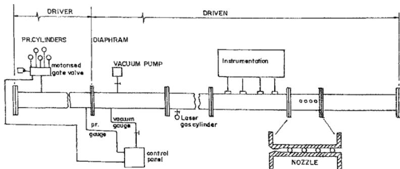
FIG. 1. Schematic diagram of shock tube-driven gasdynamic laser.
