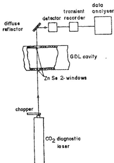
FIG. 3. Schematic diagram of small-signal gain measurement arrangement in a gasdynamic laser.
