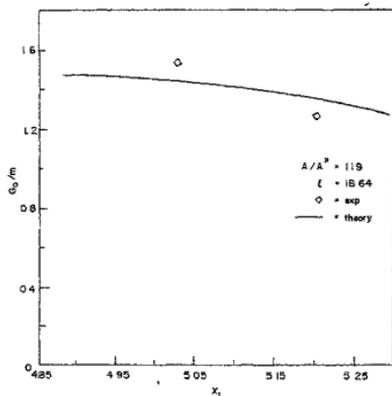
FIG. 5. Variation of small-signal gain with the universal parameter  $\chi_1$  for the composition CO<sub>2</sub>:N<sub>2</sub>:He = 11.5:50:38.5(%).
