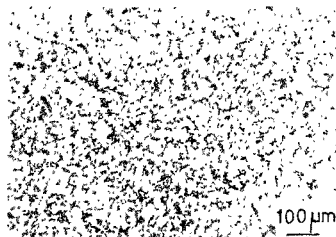
FIG. 2. Optical micrograph showing equiaxed structure in spray-formed LM6 alloy.
