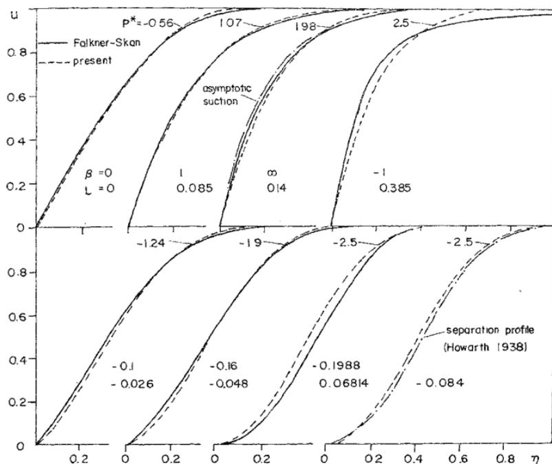
FIG. 3. Approximate representation of the Falkner-Skan profiles for various  $\beta$  and Howarth's separation profile by the proposed velocity profile (9) with the values of  $P^*$  indicated here.
