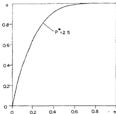
FIG. 4. Boundary-layer velocity profile (9) with  $P^* = 2.5$ . The velocity overshoot is 1.009 around  $\eta = 0.7$ .
