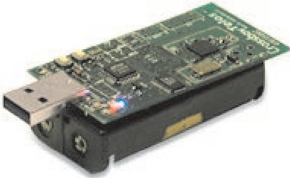
Figure 1: The Crossbow TelosB “mote” which was utilised for developing the SmartDetect WSN.
