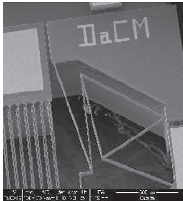
Figure 27: A close-up view of the displacement-amplifying compliant mechanism (DaCM) as fabricated in an SOIMUMPs run.
