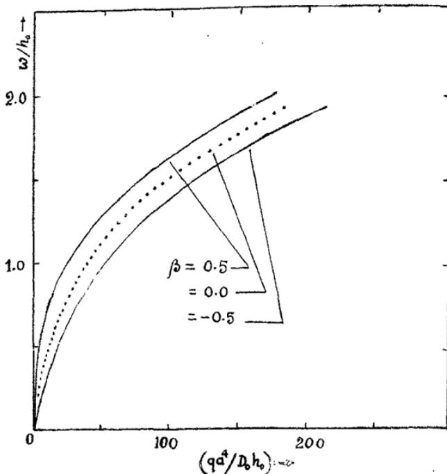
FIG. 1. Static behaviour of square plate with parabolically varying thickness.
