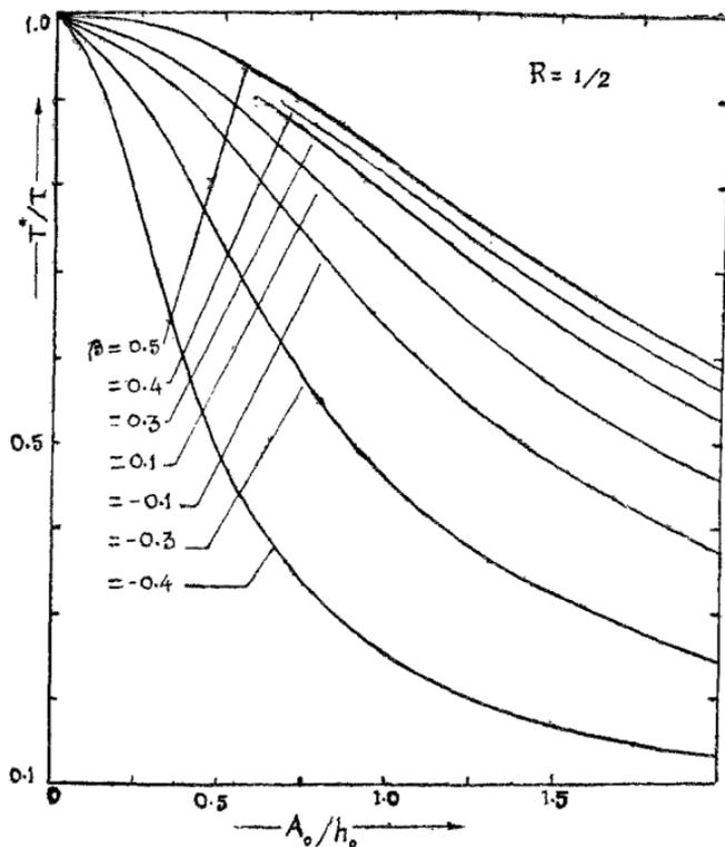
FIG. 2. Relative time period vs. relative amplitude for a rectangular plate with aspect ratio,  $1/2$ .
