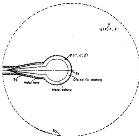
FIG. 2. Surface  $S$  used in the application of Love-Schelkunoff's equivalence principle  $S = S_1 + S_2 + S_3$ .
