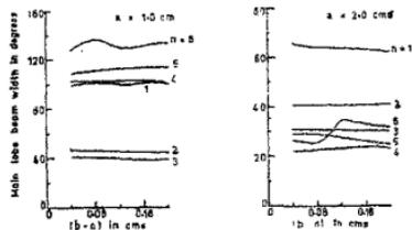
FIG. 4. Variation of main lobe beam width with coating thickness.  $f = 9.375$  GHz,  $\epsilon_r = 2.56$ ,  $\theta_1 = 130^\circ$ .
