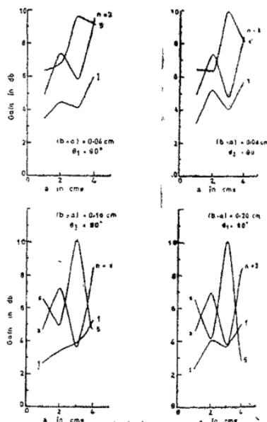
FIG. 18. Variation of gain with the inner radius ' $a$ ' for equatorial excitation,  $f = 9.375$  GHz,  $\epsilon_r = 2.56$ .
