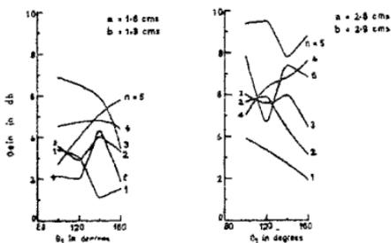
FIG. 16. Variation of gain with angle of excitation  $\theta_1$ .  $f = 9.375$  GHz,  $\epsilon_r = 2.56$ .
