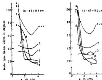
FIG. 6. Variation of the main lobe beam width with the inner radius 'a'.  $f = 9.375$  GHz,  $\epsilon_r = 2.56$ ,  $\theta_1 = 130^\circ$ .
