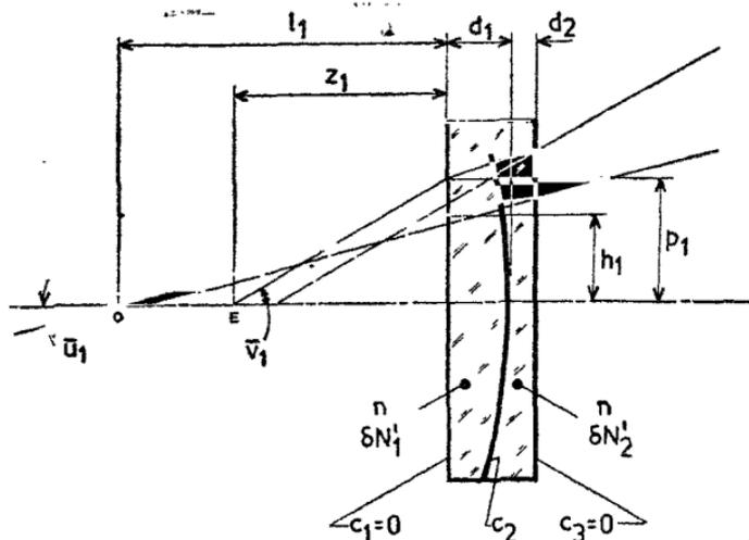
FIG. 1. Hyperchromatic doublet (System parameters and initial ray data).
