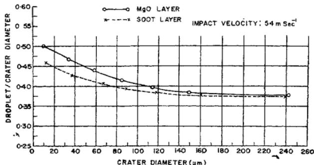
FIG. 1. Crater diameter vs droplet to crater size ratio in oxide and soot layers.
