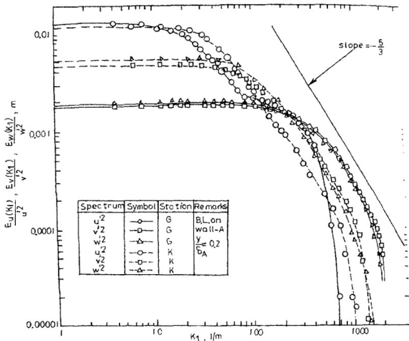
FIG. 10. Spectra of  $u'^2$ ,  $v'^2$  and  $w'^2$  in the boundary layer,  $\alpha = 0^\circ$ .
