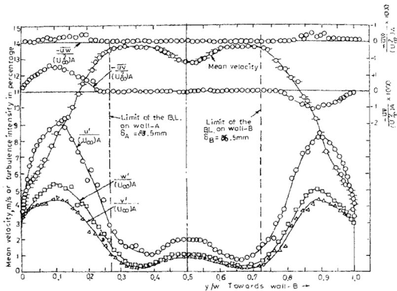
FIG. 2. Distribution of turbulence quantities at station M,  $\alpha = 0^\circ$ .
