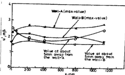
Fig. 6. Comparison of maximum  $u'$  in the boundary layer on wall-A with that on wall-B,  $\alpha = 4^\circ$ .
