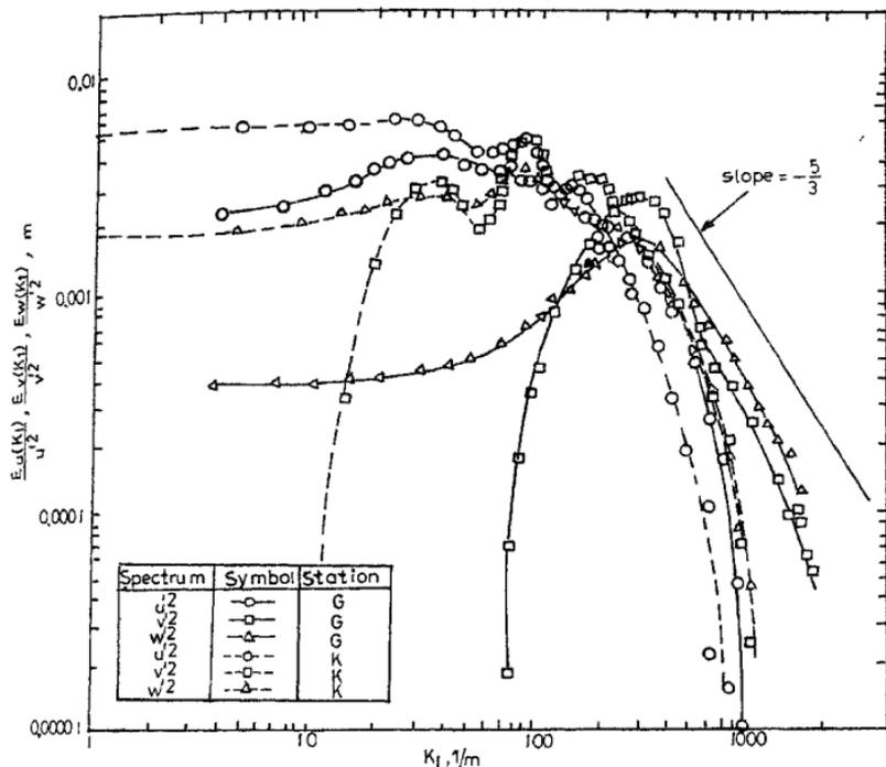
FIG. 11. Spectra of  $u'^2$ ,  $v'^2$  and  $w'^2$  along the axis of the wake,  $\alpha = 0^\circ$ .
