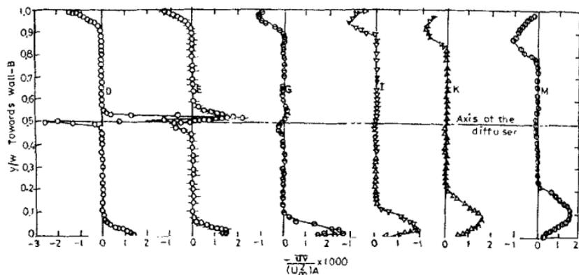
FIG. 4a. Distribution of  $\bar{u}\bar{v}$ ,  $\alpha = 0^\circ$ .
