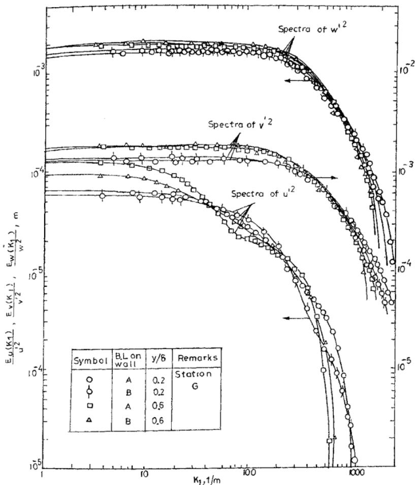
FIG. 9. Comparison of energy spectra in the boundary layer near walls-A and B,  $\alpha = 0^\circ$ .
