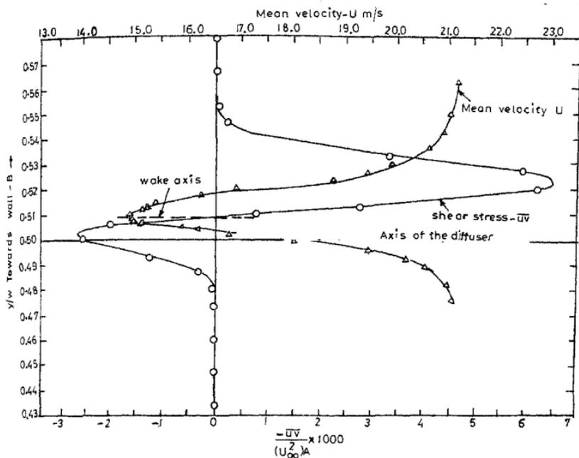
FIG. 8. Distribution of  $\overline{uv}$  and  $U$  near the axis of the wake, station D,  $\alpha = 0^\circ$ .
