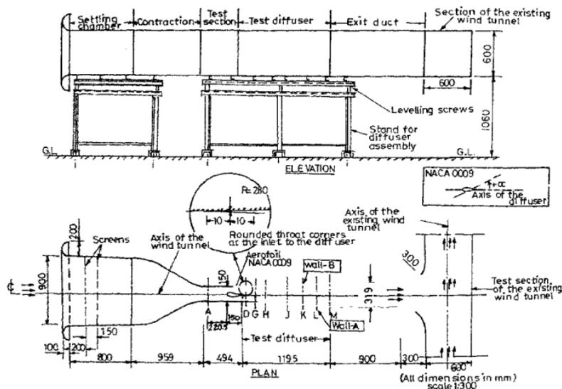
FIG. 1. Sketch of the wind tunnel.
