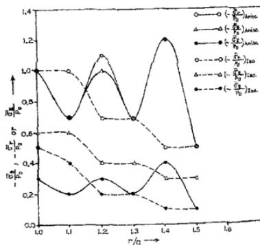
FIG. 2. Loading system II ( $p_1 = p_0/2$ ) isotropic and anisotropic variation.
