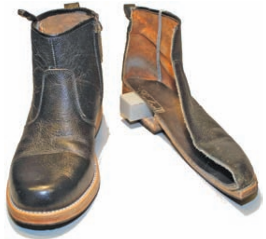
Figure 3: Shoes with the OpenShoe foot-mounted INS implementation integrated in the heels.
