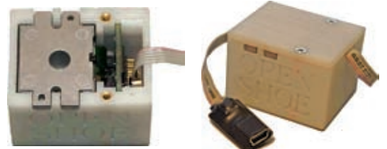
(c) The system casing body with grooves to hold the IMU and the main PCA in place.
